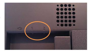
If you are using The Grid 2 there is also the option to set the user programmable buttons on the back of the Tellus 5 as switches.
