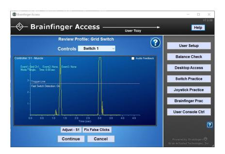
From here you can review the profile. This screen will show the muscle signal (yellow line) and you will also see that there is a Trigger line. When you carry out a muscle action (e.g. eyebrow raise, swallow, clenching teeth together etc) this needs to get above the Trigger line so that it can activate the switch press.
