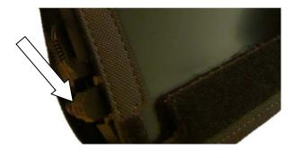
6. The PowerBox MOTION is also equipped with an active stylus. You can find the stylus in its bay by pressing the small square button on the right hand side of the device: the stylus bay will open.
