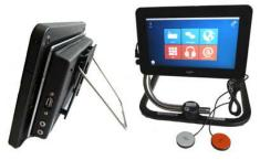
2. Turn ON the PowerBox MOTION by pressing the small square button at the top left hand side of the device.
