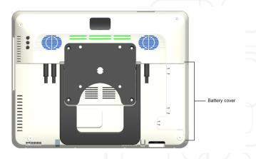
Press the two lids (1) of the battery cover downwards and slide the battery cover away from the Tellus (2).
